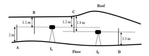
If the reduced level of station **A** is 100.0 m, the reduced level of station **D** in m is \_\_\_\_\_ (round off to 1 decimal place).
