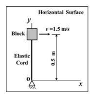
The cord hinged at  $\mathbf{O}$  is initially unstretched and always remains elastic. The block is given a velocity v of 1.5 m/s perpendicular to the cord. The magnitude of velocity in m/s of the block at the instant the cord is stretched by 0.4 m is
