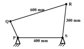
For the mechanism to be a crank-rocker mechanism, the length of the link PQ
