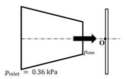
The inlet and outlet areas of the nozzle are 0.1 m<sup>2</sup> and 0.02 m<sup>2</sup>, respectively. Take air density as constant and equal to 1.2 kg/m<sup>3</sup>. If the inlet gauge pressure of air is 0.36 kPa, the gauge pressure at point **O** on the plate is \_\_\_\_\_ kPa (round off to two decimal places).
