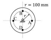
The rotor is driven by a motor at uniform angular speed of 10 rad/s. If one of the masses gets detached then the magnitude of the resultant unbalance force on the rotor is \_\_\_\_\_\_ N (round off to 2 decimal places).
