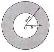
Area of the embankment (Shaded region) =  $\pi (R^2 - r^2) = \pi (10^2 - 5^2)m^2 = \frac{22}{7} \times 75 m^2$
