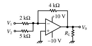
if  $V_1 = 1$  V and  $V_2 = 2$  V, the value of  $V_0$  is \_\_\_\_\_V (up to one decimal place).
