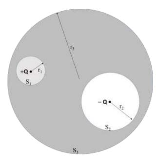
Two equal and opposite point charges + Q and - Q are located as shown in the figure above. A surface integral,  $F_i$  is defined on surface  $S_i$  of a sphere of radius  $r_i$  as follows:
