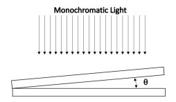
If the wavelength of light used to get a fringe spacing of 1 mm is 450 nm, the wavelength of light (in nm) to get a fringe spacing of 1.5 mm is \_\_\_\_\_
