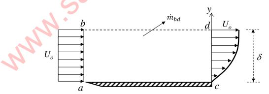
The ratio of the mass flow rate,  $\dot{m}_{bd}$ , leaving through the horizontal section b-d to that entering through the vertical section a-b is \_\_\_\_\_
