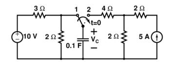
If time t is in seconds, the capacitor voltage  $V_C$  (in volts) for t > 0 is given by
