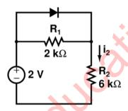
The magnitude of the current i<sub>2</sub> (in mA) is equal to \_\_\_\_\_
