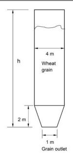
A circular grain silo with conical bottom, as shown in figure, is filled with wheat (true density 1200 kg m<sup>-3</sup>) with porosity of 0.6. Five hundred metric tonne of wheat fills 80% of its capacity (by volume). The total height (h) of the silo from its grain outlet end in m is \_\_\_\_\_\_.
