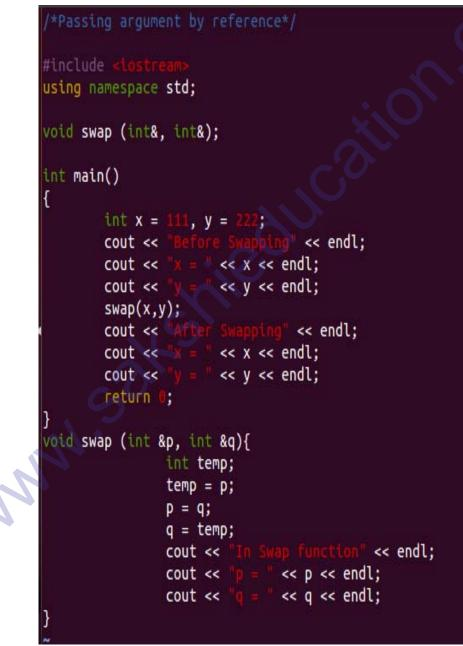
Figure3: Example program for pass by reference
