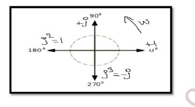
So by multiplying an imaginary number by  $j^2$  will rotate the vector by 180° anticlockwise, multiplying by  $j^3$  rotates it 270° and by  $j^4$  rotates it 360° or back to its original position. Multiplication by  $j^{10}$  or by  $j^{30}$  will cause the vector to rotate anticlockwise by the appropriate amount. In each successive rotation, the magnitude of the vector always remains the same.
