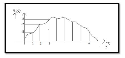
The given alternating current wave is divided into n equal number of time intervals. Let the mean value of the current during the intervals  $be_{i_1,i_2} - - - i_n$ . Let this current be allowed through a circuit having resistance R. Then the average power dissipated by the resistor in the interval is
