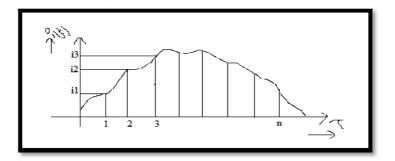
The average value of an alternating current is defined as that value of the steady current which transfers the same amount of charge across any circuit as is transferred by the given AC current in the same circuit for same time. For the alternating current for above fig, the average value is:
