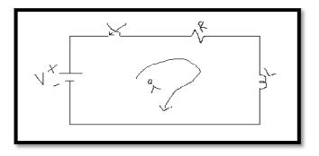
Consider a circuit consisting of a resistance and inductance as shown in fig. the inductor in the circuit is initially uncharged and is in series with the resistor. When switch S is closed, we can find the complete solution for current. Application of Kirchoff's law to the circuit results in fallowing differential equations.
