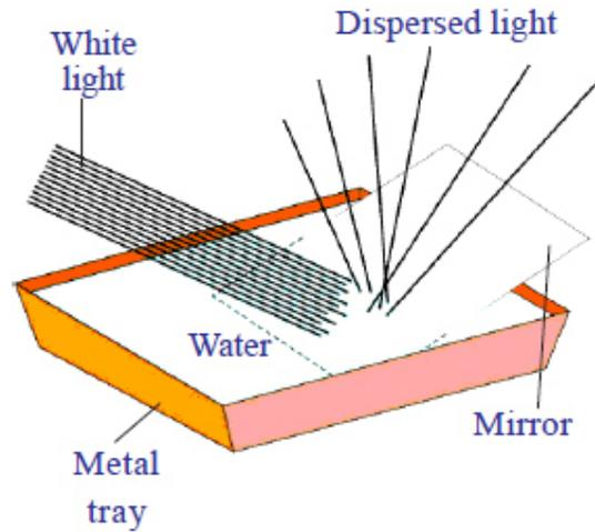
**9. Prism used in binoculars. Collects information why prisms are used in binoculars (AS<sub>4</sub>)**
