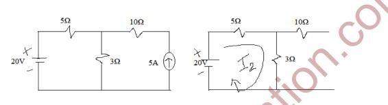
According to the superposition theorem, the current I2 due to the 20V voltage source with 5A source open circuited = 20/(5 + 3) = 2.5A
