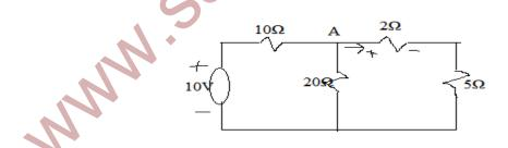
Assuming a voltage V at node A as shown, the current equation is,
