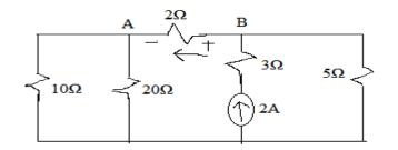
The current in the 2  $\Omega$  resistor = 2 \* (5/5+8.67) = 10/13.67 = 0.73A
