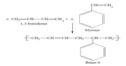
In Buna-S, 'Bu' stands for butadiene, 'na' for the symbol of sodium (Na), which is a polymerising agent, and 'S' stands for styrene. Buna-S is generally compounded with carbon black and vulcanised with sulphur. It is used in manufacturing footwear components, motor tyres and other mechanical rubber goods.
