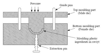
Fig. 3.5 Compressing moulding plastics
