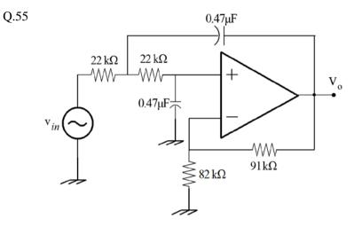
For the given low-pass circuit shown in the figure, the cutoff frequency in Hz will be \_
