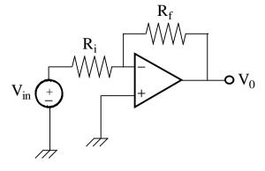
(A)  $R_i$ = 500 k $\Omega$ ,  $R_f$  = 50 k $\Omega$
