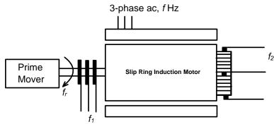
If the rotor winding is open circuited and the system is made to run at rotational speed  $f_r$  with the help of prime-mover in anti-clockwise direction, then the frequency of voltage across slip rings is  $f_1$  and frequency of voltage across commutator brushes is  $f_2$ . The values of  $f_1$  and  $f_2$  respectively are
