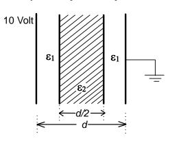
If the potential difference between one of the plates and the nearest surface of dielectric interface is 2 Volts, then the ratio  $\varepsilon_1$ :  $\varepsilon_2$  is
