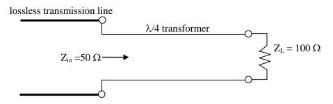
The characteristic impedance (in  $\Omega$ ) of the  $\lambda/4$  transformer is \_\_\_\_\_
