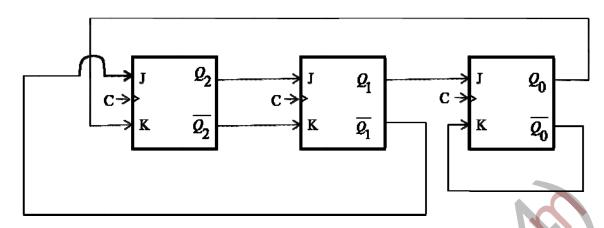
The above synchronous sequential circuit built using JK flip-flops is initialized with  $Q_2Q_1Q_0=000$ . The state sequence for this circuit for the next 3 clock cycles is
