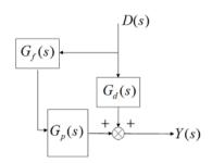
The transfer function of the process is  $G_p = \frac{5}{s+1}$  and the disturbance transfer function is
