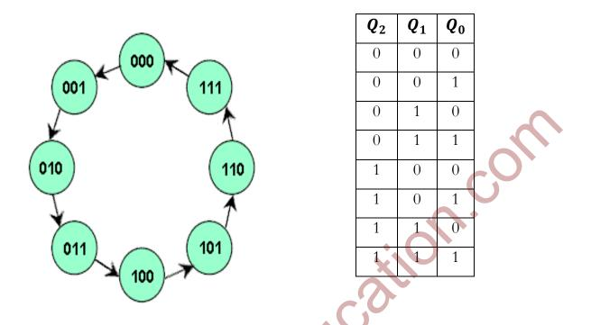
In the given count sequence, we find that flip-flop FF0 toggles with every clock pulse, flip-flop FF1 toggles only when the output of FF0,  $Q_0$  is in the '1' state, flip-flop FF2 toggles only with those clock pulses when the outputs of FF0 and FF1 are both in the logic '1' state. Such logic can be easily implemented with AND gates.
