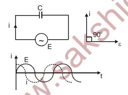
13. Purely capacitive circuit: A circuit containing an A.C source and a capacitor is known as purely capacitive circuit. If  $\varepsilon = \varepsilon_0 \sin \omega t$ , the circuit equation is
