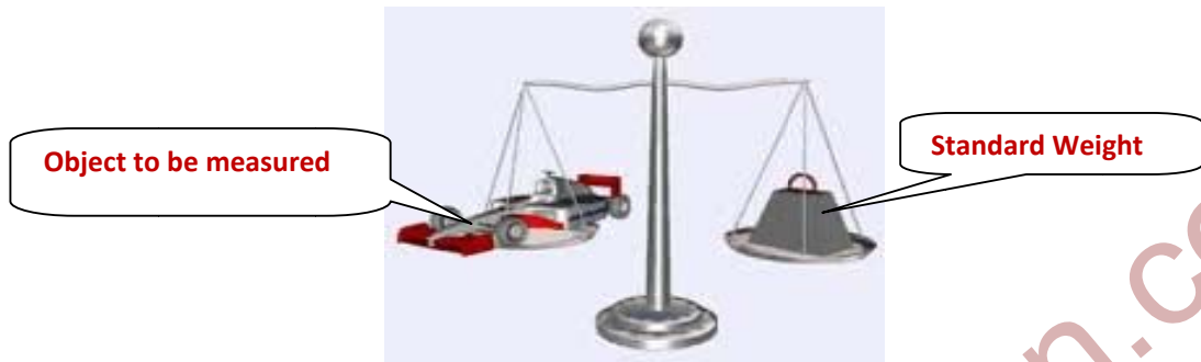
Figure 5: Simple balance with standard weight and component to be measured
