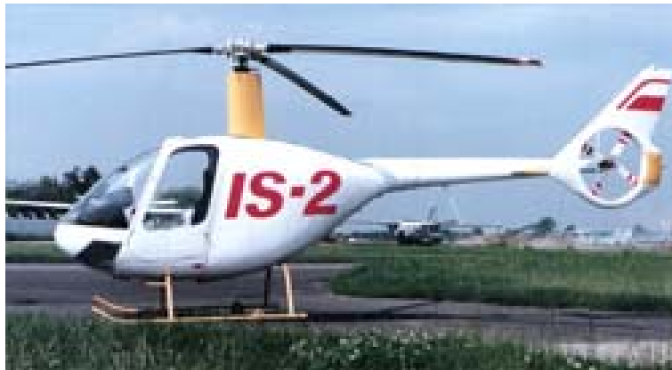
Figure 4: IS-2 Helicopter with four rotor blades of Aerofoil shape
