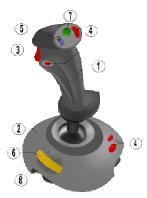
is controlling. Joysticks are often used to control video games, and usually have one or more push-buttons whose state can also be read by the computer. Figure of Joystick is shown here with description of Buttons.
