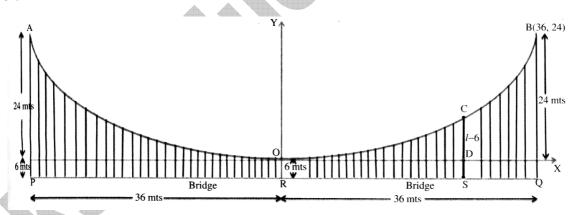
Let AOB be the cable [O is its lowest point and A, B are the highest points]. Let PRQ be the suspension bridge suspended with PR = RQ = 36 mts.
