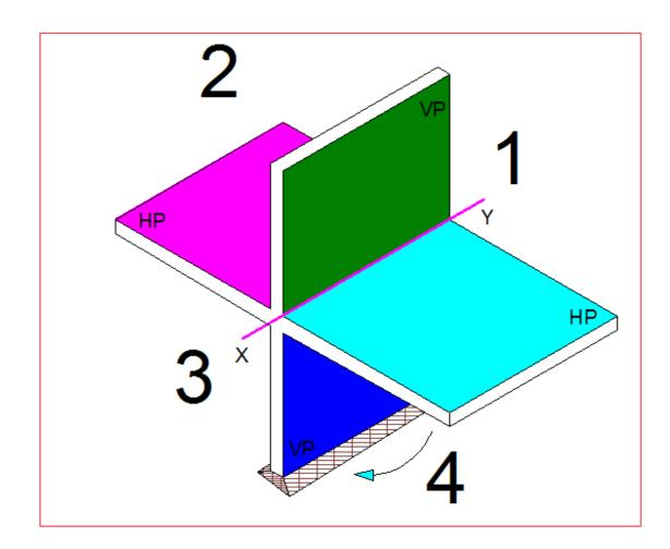
**First quadrant ---** Above HP and in front of VP **Second quadrant ---** Above HP and behind VP **Third quadrant ---** Below HP and behind VP **Fourth quadrant ---** Below HP and in front of VP
