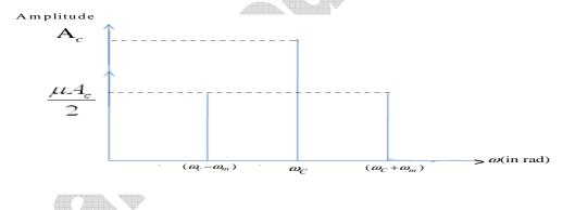
As long as the broadcast frequencies are sufficiently space out so that sidebands do not overlap, different stations can operate without interfering with each other.
