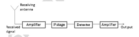
The IF signal contains the frequencies  $\omega_c$  and  $\omega_c \pm \omega_m$ . To obtain original message signal m(t) of angular frequency  $\omega_m$ , simple AM detector is shown in diagram.
