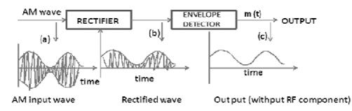
The modulated signal of the form given in (a) of fig is passed through a rectifier to produce the output shown in (b). This envelope of signal (b) is the message signal. In order to retrieve m (t), the signal is passed through an envelope detector (which may consist of a simple RC circuit).
