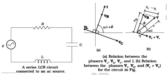
Let  $i = i_0 \sin(\omega t + \phi)$  be ac current in each element at any time where  $\phi$  is the phase difference between voltage of source and the current in the circuit. Let  $V_L, V_R, V_C$  and V represent the voltage across the inductor, resistor, capacitor and the source respectively which are shown in the phasor.
