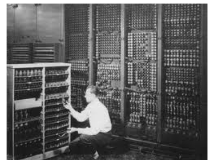
Replacing a bad tube means checking among ENIAC's 15000 possibilities.
