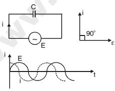
13. **Purely capacitive circuit:** A circuit containing an A.C source and a capacitor is known as purely capacitive circuit. If  $\varepsilon = \varepsilon_0 \sin \omega t$ , the circuit equation is  $Q = c\varepsilon = c\varepsilon_0 \sin \omega t$  by differentiating;
