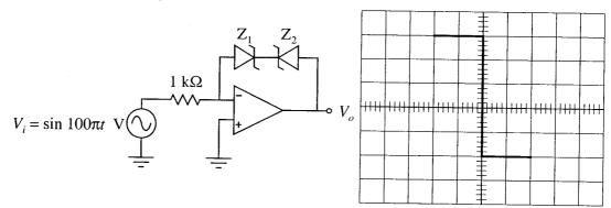
Assuming that the opamp is ideal and the zener diodes have forward biased voltage drop of 0.7 V, the values of reverse break-down voltages of  $Z_1$  and  $Z_2$  are, respectively,
