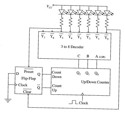
Assuming that the initial value of counter output  $(Q_2 \ Q_1 \ Q_0)$  as zero, the counter outputs in decimal for 12 clock cycles are
