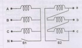
The star-delta transformer shown above is excited on the star side with a balanced, 4-wire, 3-phase, sinusoidal voltage supply of rated magnitude. The transformer is under no load condition.
