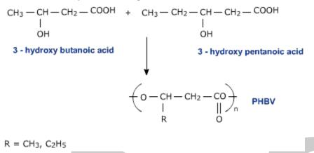
The properties of PHBV vary according to the ratio of both the acids.
