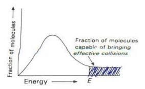
In the graph 'E' corresponds to minimum or threshold energy for effective collision in a hypothetical reaction.
